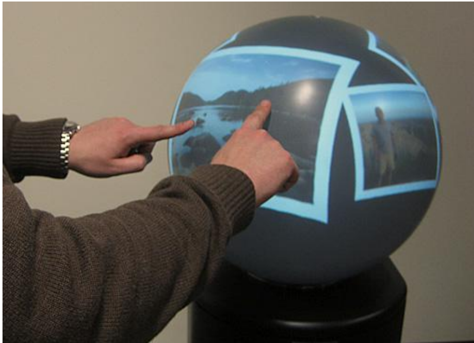
Figure 2.12: The Sphere provides a touch-sensitive display on the surface of a sphere. Image courtesy of Hrvoje Benko.
