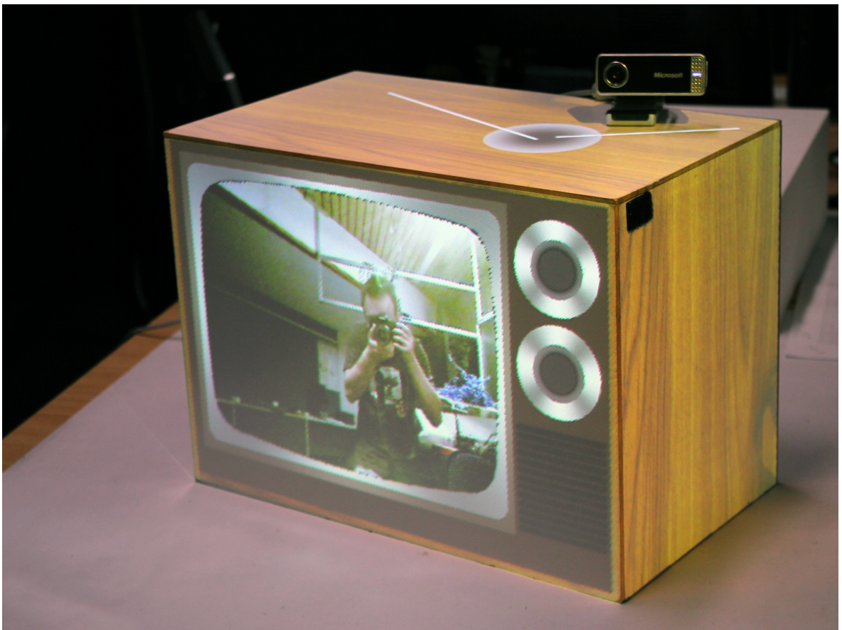
Figure 7.4: Result of running the TV module. A textured 3D model is projected onto a blank white box. The video stream is captured from the attached webcam and displayed on the TV.
