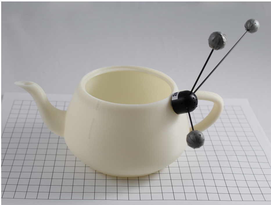
Figure 2.14: Tracking systems such as those from Optitrack use retro-reflective markers to track the position and orientation of objects.
