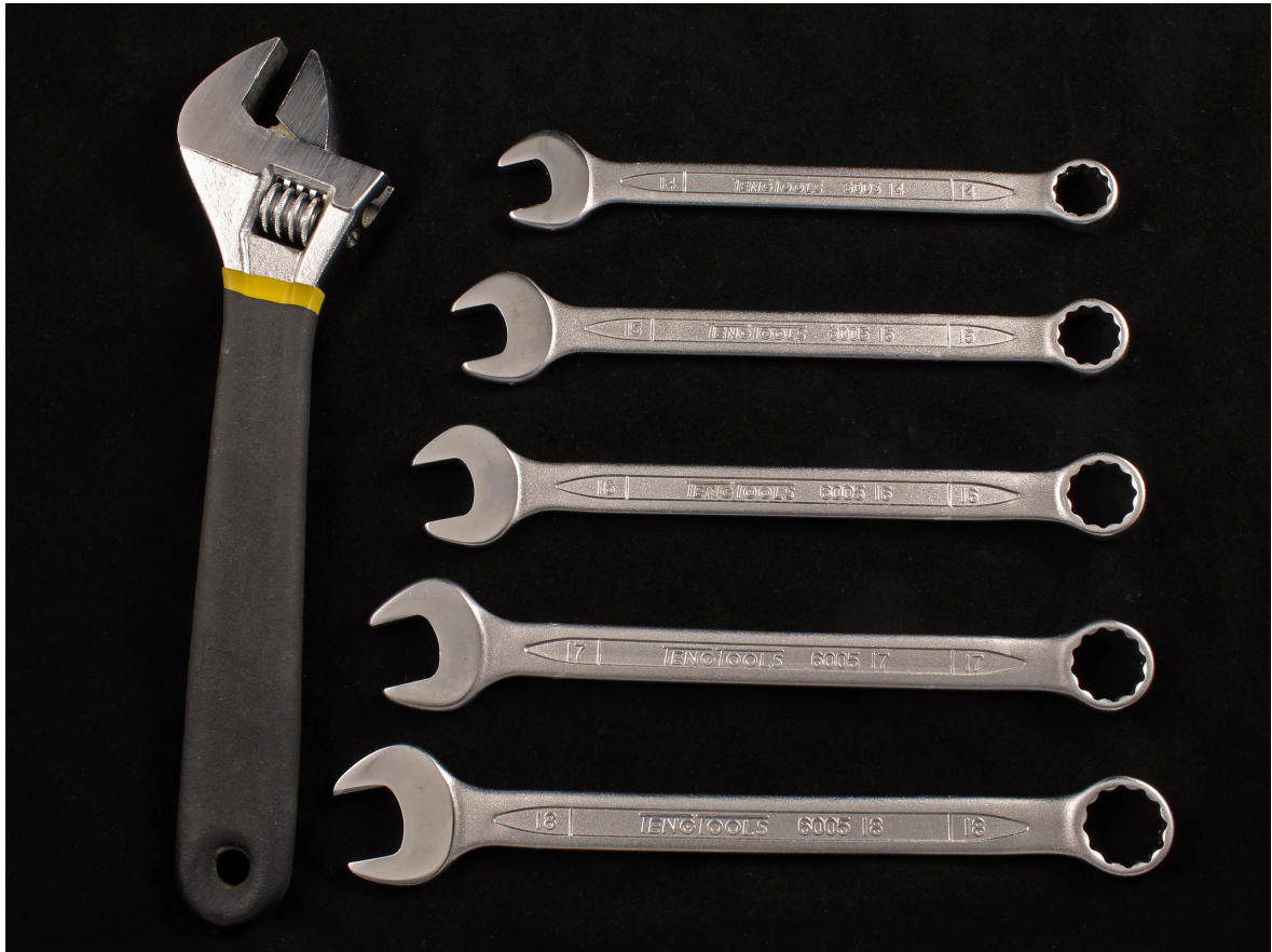
Figure 3.1: A mechanic can choose between several single sized wrenches, or a shifting spanner which works with any size.
