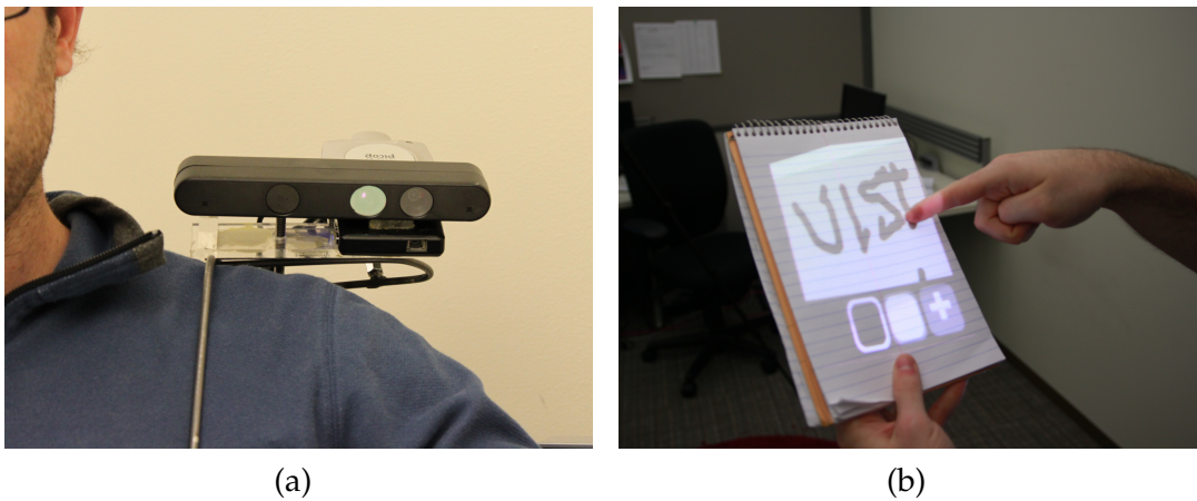
Figure 2.9: (a) OmniTouch incorporates a shoulder mounted projector and depth sensor. (b) The depth sensor is used to detect projection surfaces and allow interaction. Images courtesy of Chris Harrison.
